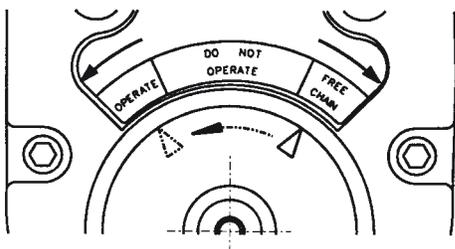
7. Pull sharply on the loose end of chain and **THEN LET GO OF CHAIN.** Pull sharply on the lower hook side of chain, to make sure gearing is fully engaged.
