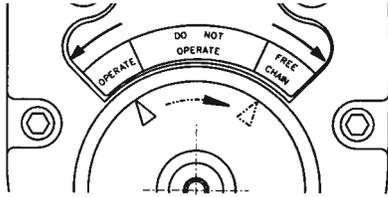
4. Pull on hook side and loose end side of load chain to make sure chain feeds freely into and out of the hoist.
