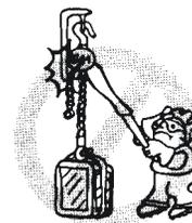
Do not operate with Puller frame resting against any object. Apply the load gently. Do not jerk it.
