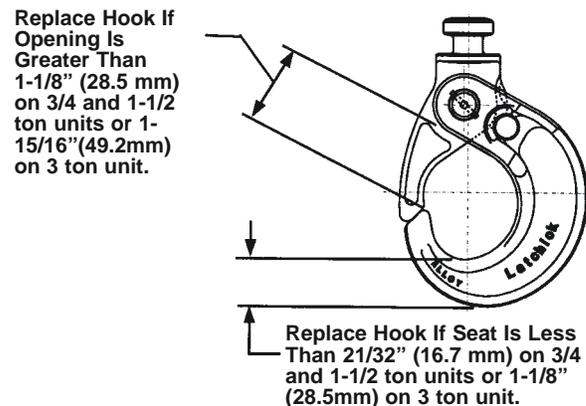
On Latchlok type hooks, measure seat wear and throat opening as shown above and replace hook if measurements indicate the need to do same.
