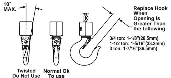
On latch type hooks, check to make sure that the latch is not damaged or bent and that it operates properly with sufficient spring pressure to keep the latch tightly against the tip of the hook and allow the latch to spring back to the tip when released. If the latch does not operate properly, it must be replaced. See above illustrations to determine when the hook must be replaced.
