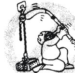
Never use an extension on the lever! You're dangerously overloading the Puller if you exceed the rated lever pull or if you have to use a lever extension to lift or pull a load.
