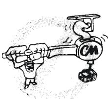
Using the upper hook, attach the hoist to support.
