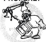
Be sure the Short Handle Puller and load are in a straight line. Do not use unless frame and chain form a straight line between hooks.
