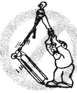
Be sure load is hooked securely. Do not tip load the hook. Do not load hook latch. Hook latch is to prevent detachment of load under slack chain conditions only.
