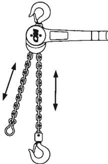
5. Grasp unit by frame or upper hook and pull on end ring or lower hook to pull the chain through hoist to the length required to attach lower hook to load. Pull on end ring to take-up slack in chain and **THEN LET GO OF END RING.**
